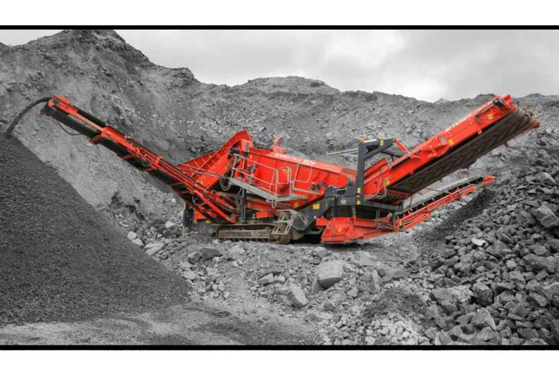
The fourth generation Terex Finlay 883+ has been developed as a high capacity and versatile heavy duty scalper to work in primary and secondary screening applications such as quarry and mining, iron ore, construction demolition waste, sand, gravel, compost, top soil and coal.
