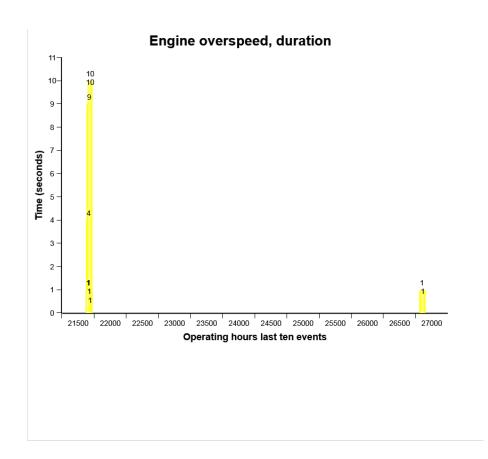
The diagram shows how long time in seconds that the engine speed has exceeded 2200 rpm (overspeed) the last ten times related to the total operating hours when it occurred.
