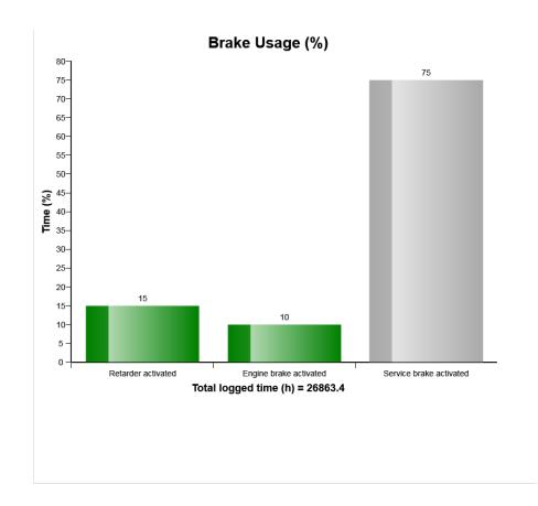
The diagram shows the total time for activated retarder, engine brake and the total time for activated service brake (exceeding 4 bar).
