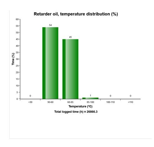
The graph shows the time distribution of the temperature, while engine running.
