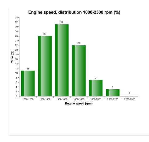
The diagram shows the percentage distribution that the engine has operated in various engine speed ranges between 1000 and 2300 rpm.
