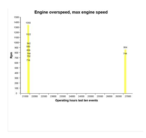
The diagram shows the maximum engine-speed the last ten times the engine have exceeded 2200 rpm (over-speed)
