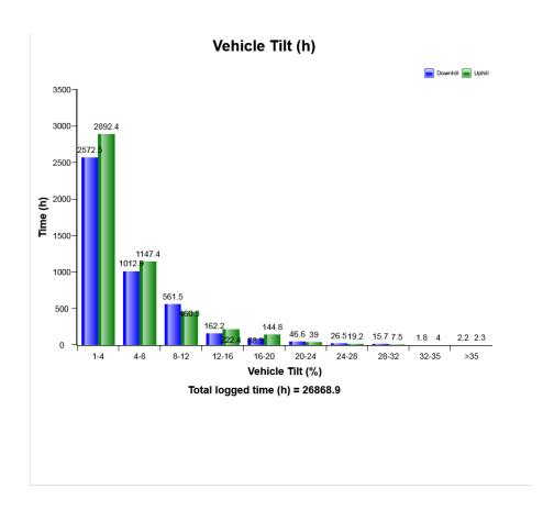
The diagram shows the distribution of the longitudinal tilt in percent (not degrees), the criteria to get registrations is that the vehicle speed exceeds 1 km/h (0,62mph) and that the engine is on.
