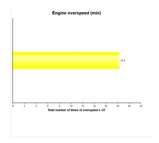
The diagram shows how long time in minutes that the engine-speed has exceeded 2200 rpm. Information regarding how many times the engine speed has been above 2200 rpm is noted below the diagram.
