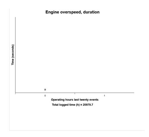
The diagram shows how long time in seconds that the engine speed has exceeded 2200 rpm (A35E) or 2100 rpm (A40E) (over-speed) the last twenty times related to the total operating hours when it occurred.
