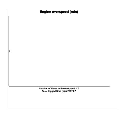
The diagram shows how long time in minutes that the engine-speed has exceeded 2200 rpm for A35E or 2100 rpm for A40E. Information regarding how many times the engine speed has been above 2200 or 2100 rpm is noted below the diagram.
