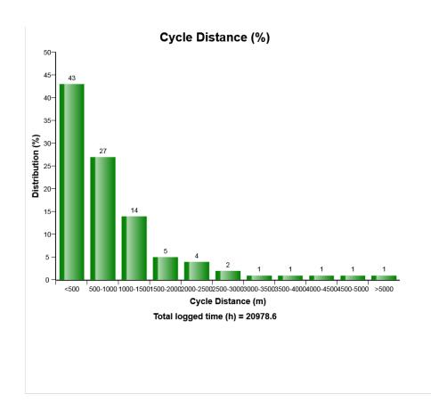
The diagram shows the distribution of the working cycle distance. The distance driven between 2 valid cycle registrations.
