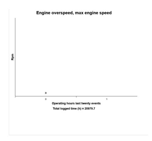
The diagram shows the maximum engine-speed the last twenty times the engine have exceeded 2200 rpm (A35E) or 2100 rpm (A40E) (over-speed)
