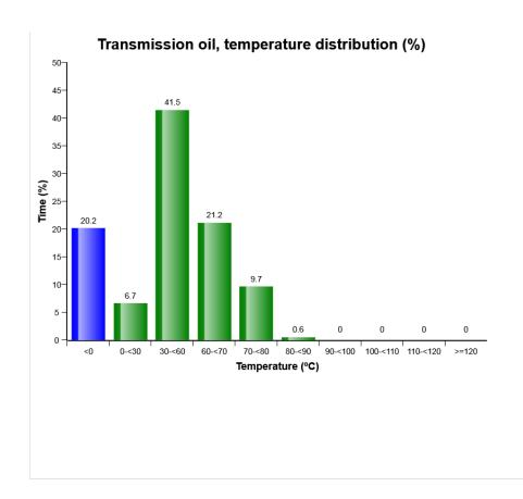
The diagram shows the transmission oil temperature in various temperature ranges. The time is displayed in the following ten temperature ranges:
