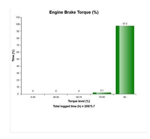
The diagram shows the Engine Brake usage in terms of percent up to maximum torque.
