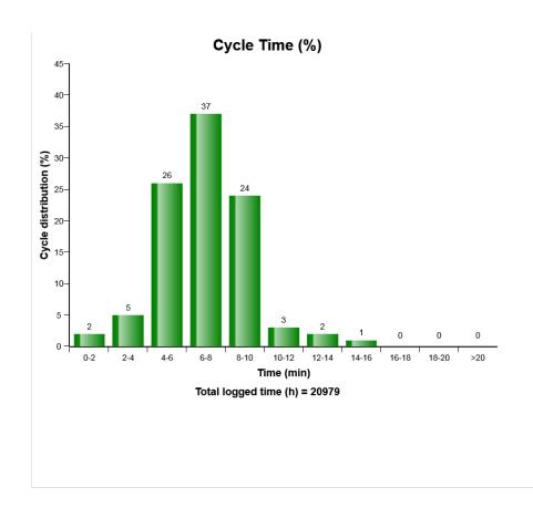
The diagram shows the distribution of the working cycle time. The time between 2 valid cycle registrations is registered. Time starts from lifting the body.
