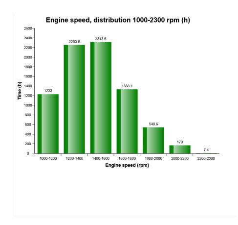
The diagram shows the time that the engine has operated in various engine speed ranges between 1000 and 2300 rpm.
