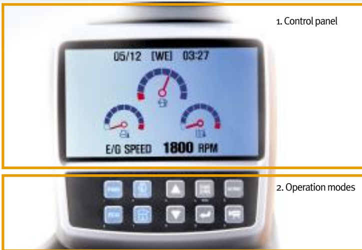
Control stand (Telescopic Function)
