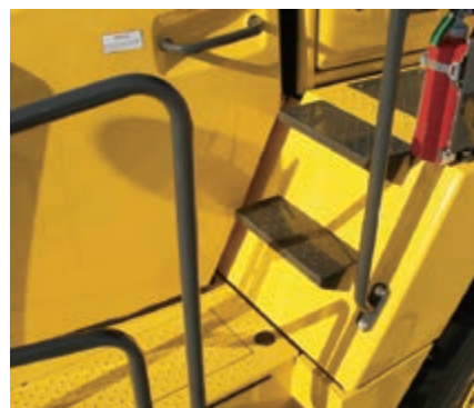
Safe cab access with handrail, away from the potentially hazardous articulation
