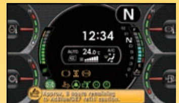
AdBlue® level and refill guidance
