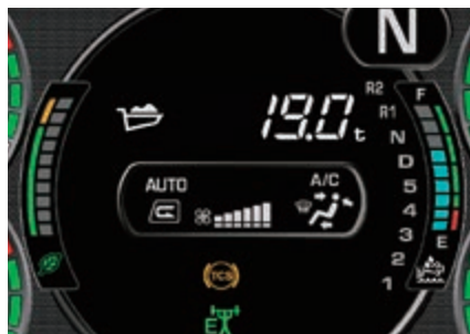
Payload meter displays the loaded weight
