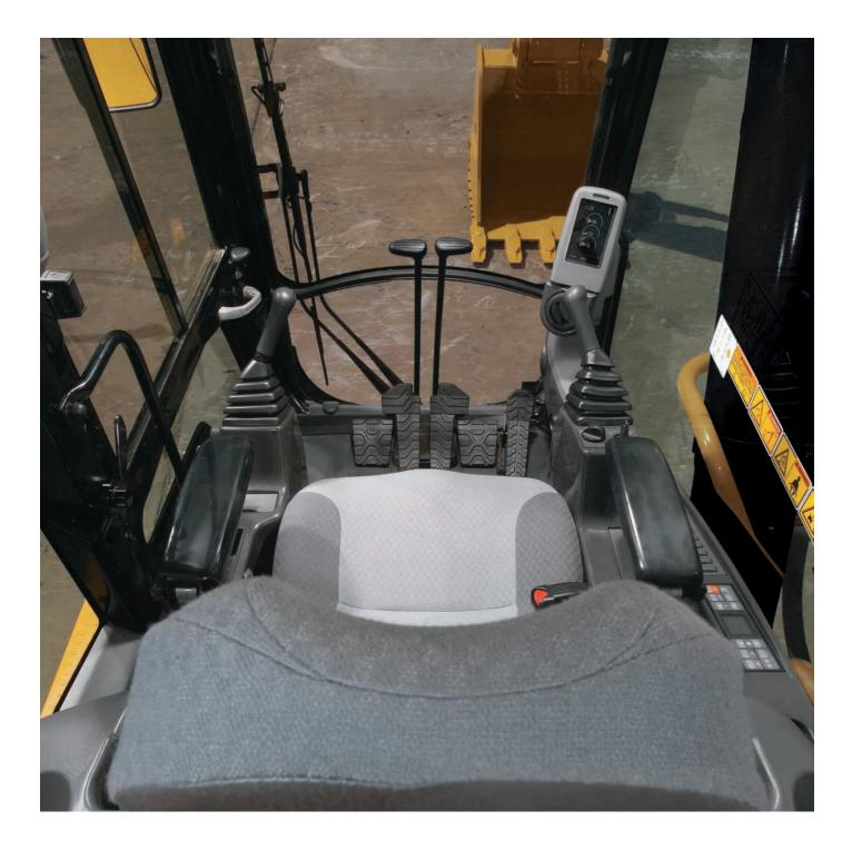
**Cab Design.** The workstation has been designed to be spacious, quiet and comfortable for the operator, assuring high productivity throughout the entire workday. Switches are conveniently located for easy access. The new monitor is located to provide excellent visibility and access.
