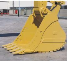
**Ground Engaging Tools.** Caterpillar Ground Engaging Tools (GET) include a variety of side cutters, sidebar protectors, and tip options to match operating conditions.
