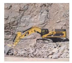
**PPPC Hydraulics.** Load sensing, Proportional Priority Pressure Compensation (PPPC) system, with Caterpillar-developed electronic actuation, provides high efficiency and excellent controllability.
