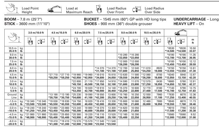
\* Limited to hydraulic capacity rather than tipping load. The above loads are in compliance with hydraulic excavator lift capacity rating standard SAE J/ISO 10567. They do not exceed 87% of hydraulic lifting capacity or 75% of tipping capacity. Weight of all lifting accessories must be deducted from the above lifting capacities.
