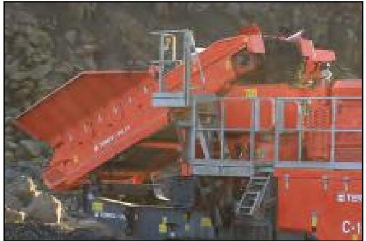
Hopper and Feeder
