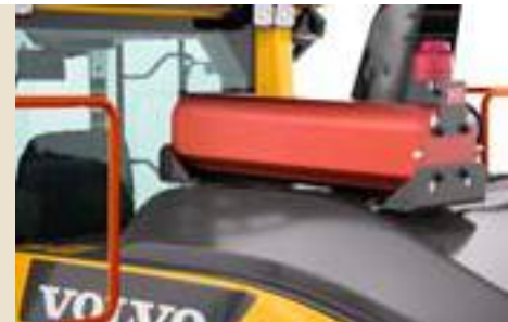
Fire suppression system
