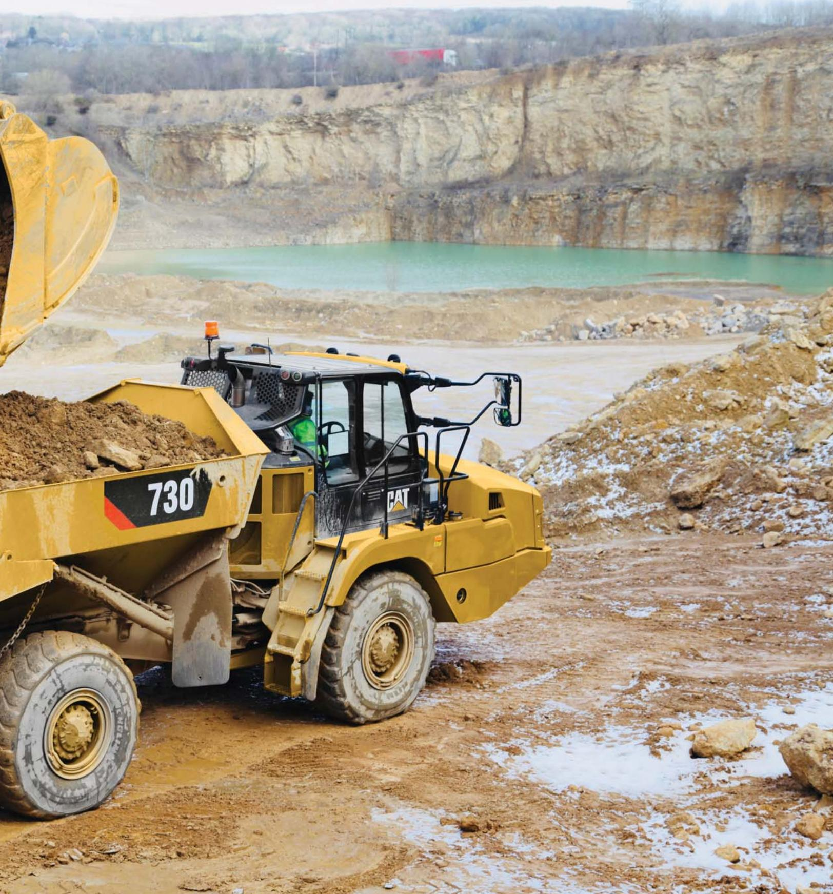
**The Cat 730 with a 17.5 m<sup>3</sup> (23 yd<sup>3</sup>)/28 tonnes (31 tons) capacity, offers demonstrated reliability and durability, high performance and productivity and a new world-class cab to improve operator comfort and ease of operation.**
