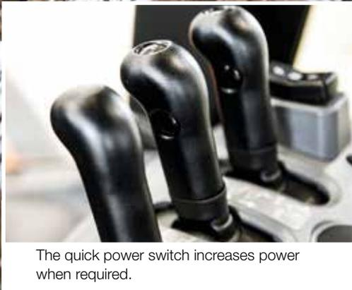
The quick power switch increases power when required.
